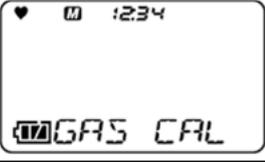
The LCD display shows a heart icon, a battery level indicator, and the number 1234 at the top. Below that, the words "GAS CAL" are displayed in a large, stylized font.    | P. 42                |
